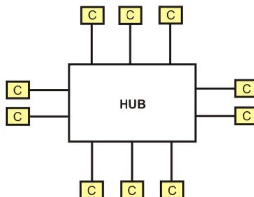
Figure 5.3.5 Interfacing a computer in 10Base-T standard
